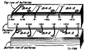
FIGURE 11.—Box BX-12, terminal strip-battery, BA-2 connections.
